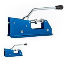
The Roll-Line® Bearing Press is perfect for the extraction and insertion of bearings from, and into the wheels. The bearing press can be transported with you in your Roll Line trolley, or mounted on a workstation. Can be used with wheels up to 70mm in diameter, and with either 7mm or 8mm bearings. With the attached hook, the bearing press can also be used to extract bearings.
