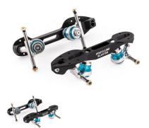
The frame (plate) Blaster is the Roller Derby version of one of the most popular Roll-Line® frames and can be used by all team members (Blocker, Jammer, Pivot). Frame derived from a drawn Aluminum bar, and completely created using computer numerical control (CNC) machining. 13 mm king-pins inclined to 16° with traditional trim. Elastomer cushions available in 5 hardnesses (colors). Aluminum trucks with 8mm steel axles and adjustable pivot pin. Toestop and tool kit included.
